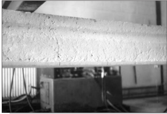
Figure 4.14: Flexural cracking in hollow core slab.
