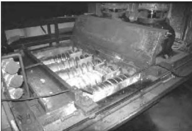
Figure 2.5: Rotating augers create forced extrusion of concrete.
